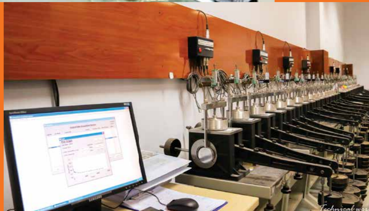
Consolidation test integrated with the Automatic Data Acquisition System
